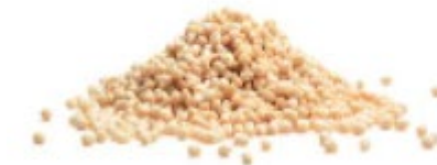
UPM Formi 3D printing material is sold as granulates. Photo: UPM
