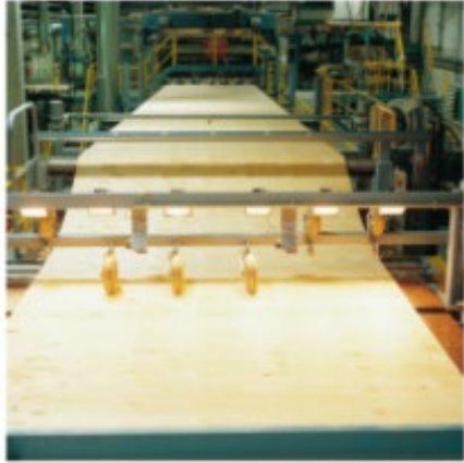
Cutting WISA spruce plywood at Pellosniemi plywood mill. Photo: UPM
